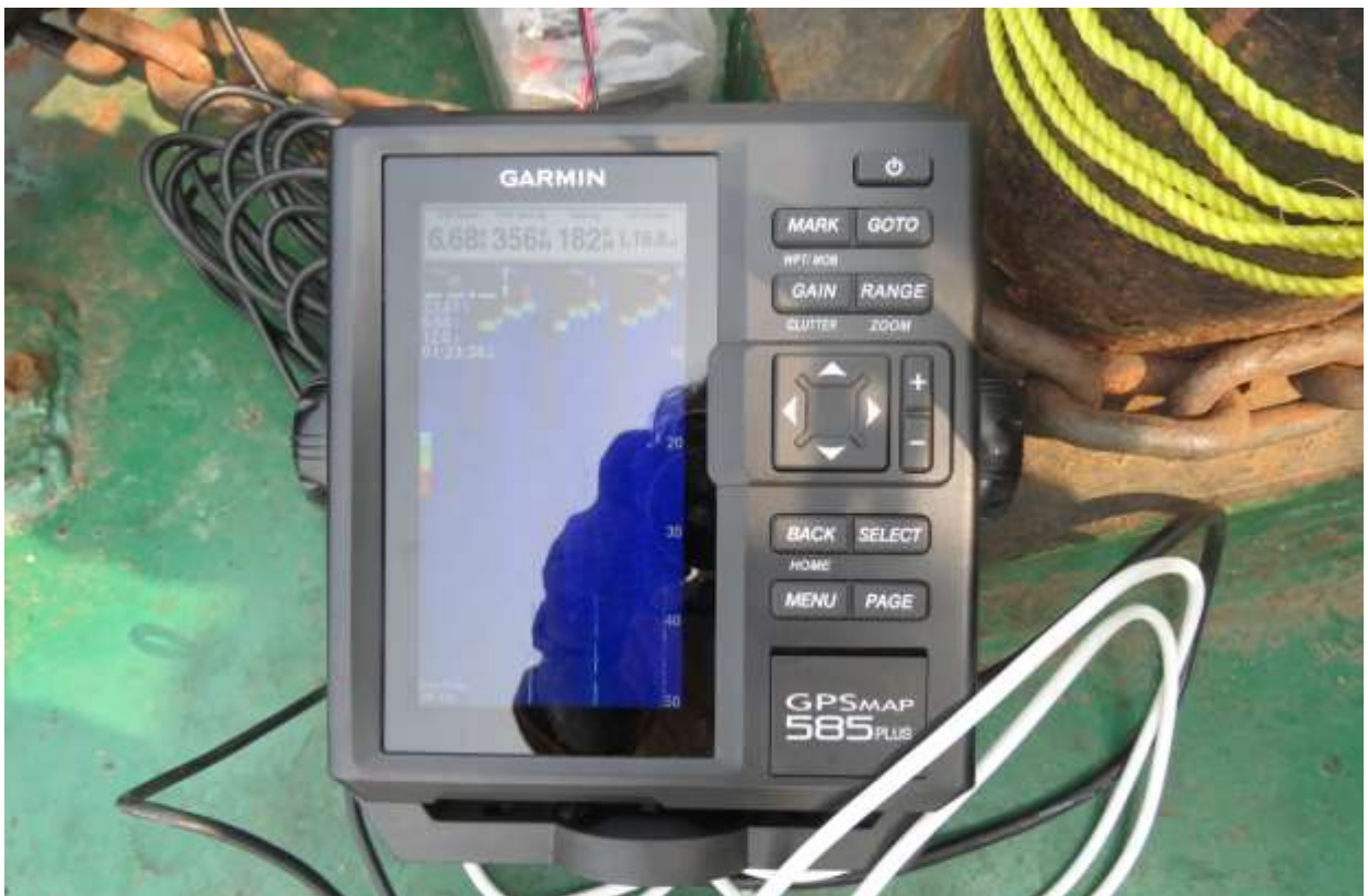
Plate9 &10 – Bathymetry Survey going on with GPS and Echo Sounder
